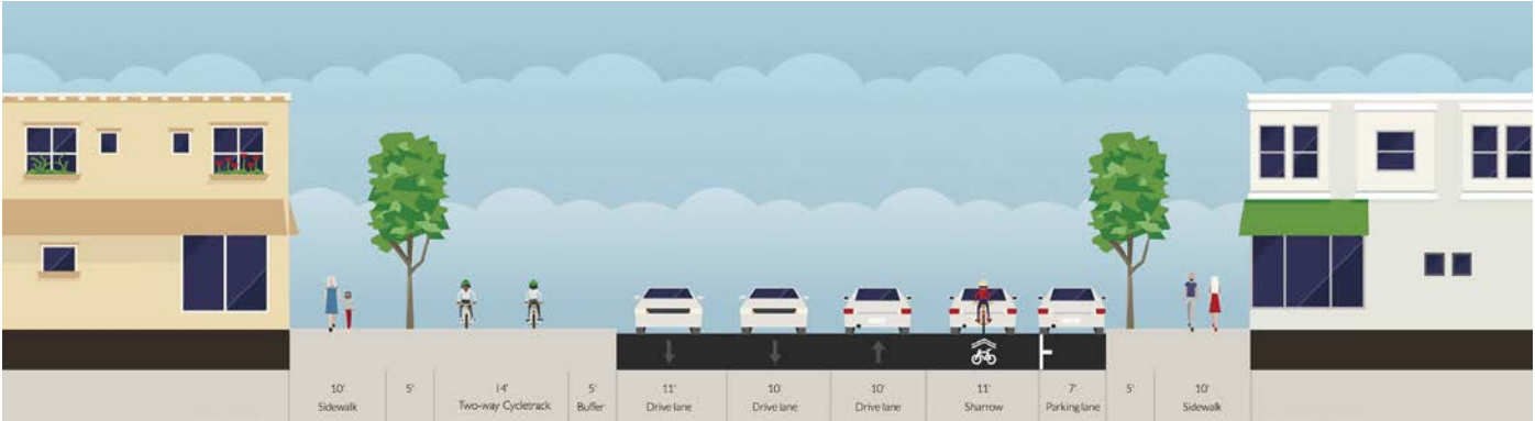
A1 - 4 LANE with CYCLETRACK (TWO-WAY)
