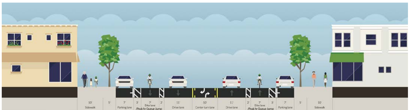
C3 - 4 LANE with BUFFERED BIKE LANES
